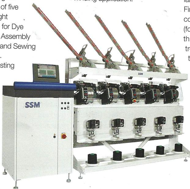
From SSM GIUDICI came the DP5-T which was exhibited in a special single-execution showing fancyflex™ for the production of slubs and thick & thin fancy yarns which gained a large interest.
